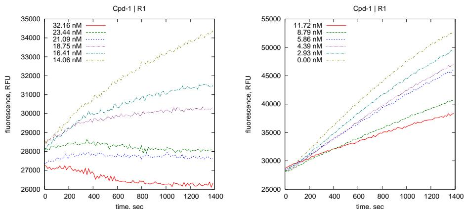
**Figure 4:** Example of anomalous (outlier) progress curve: Compound **1**, Replicate 1,  $[I]_0 = 32.16 \text{ nM}$  (bottom curve in the left-hand panel).
